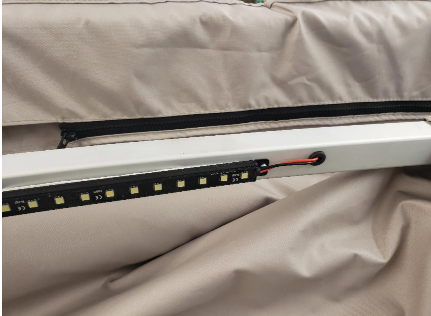
LED light wire routing in 2 nd arch
