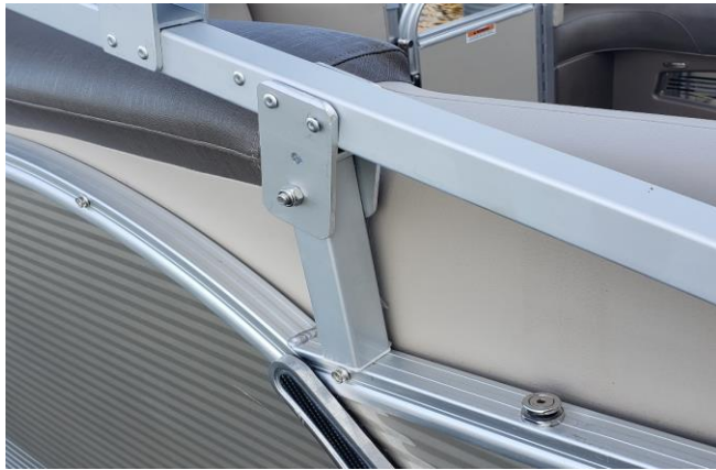
Rear support foot mounted on autobimini aluminum 4 th riser and positioned to avoid interference with boat upholstery.
