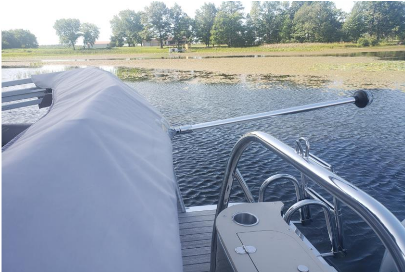
Navigation light installed on 4 th arch. Access holes are built into canvas and boot
