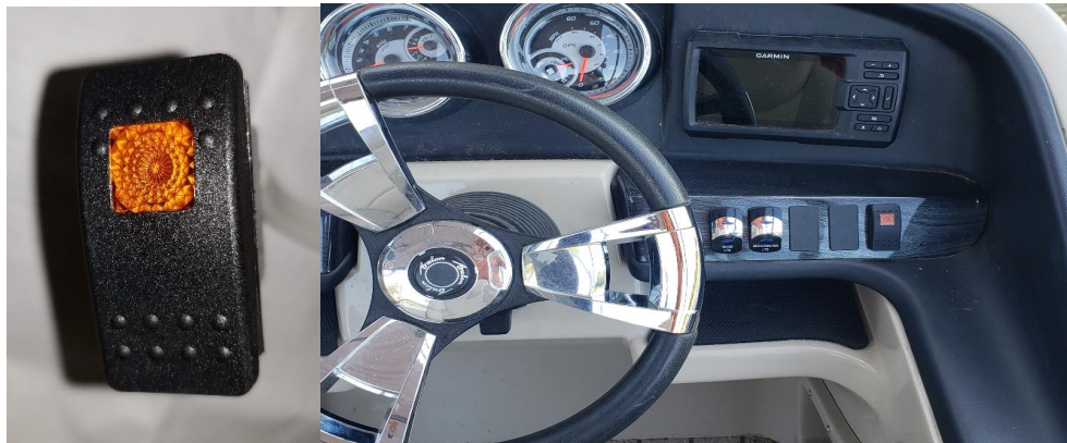
autobimini console switch; console switch installed in helm control panel
