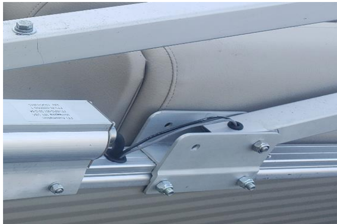
Navigation wires routed in rear riser, rear arch bracket and actuator grommet
