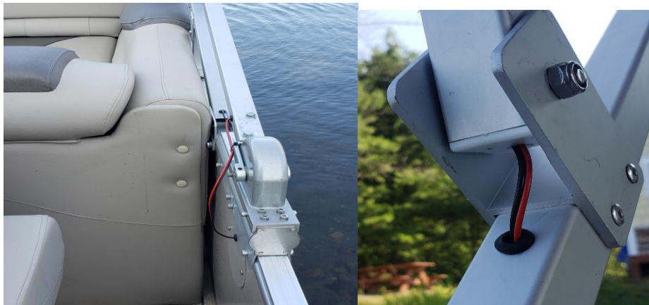
Routing of LED wire through aluminum frame
