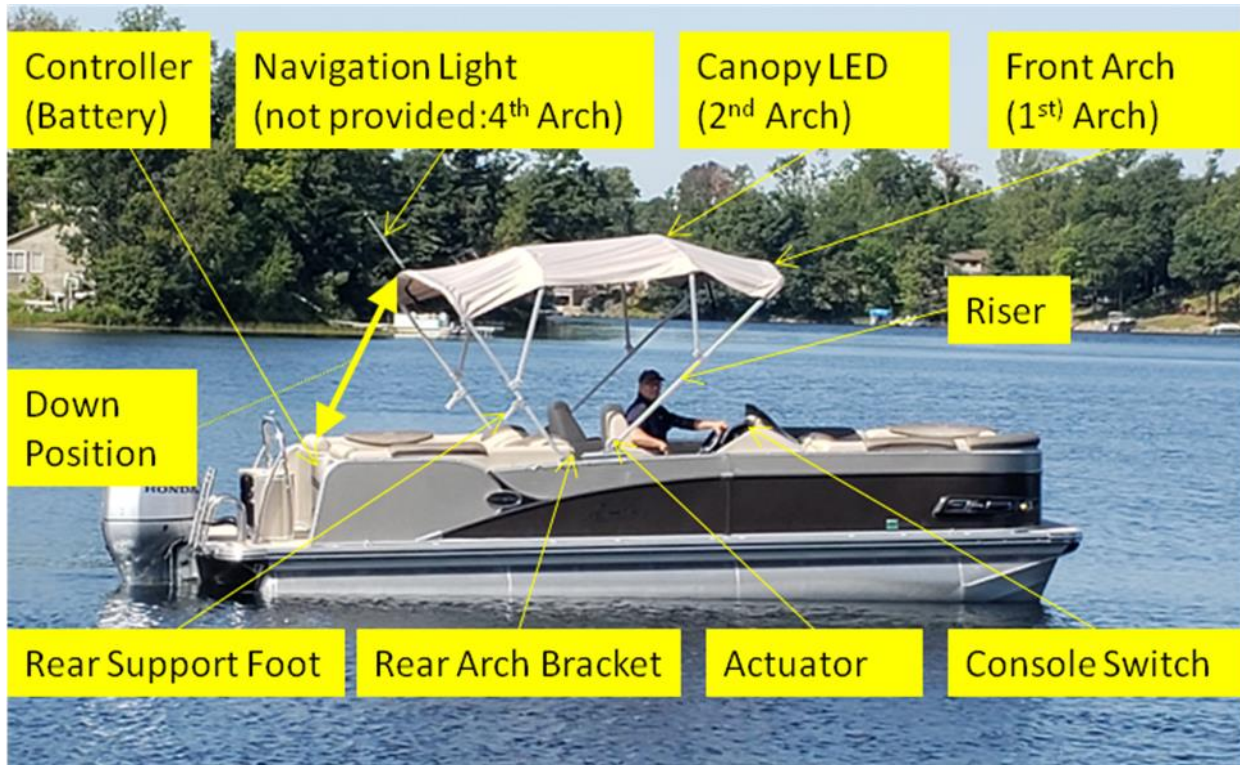
autobimini completed installation with component names and relative locations
