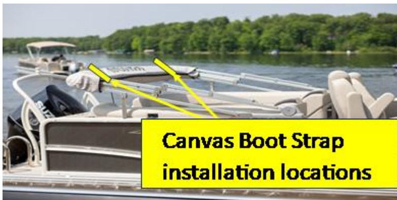
Canvas Boot Strap installation location (secures frame/boot for high-speed travel)
