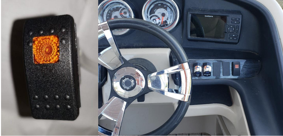
autobimini console switch (left) and console switch installed in helm control panel (right)
